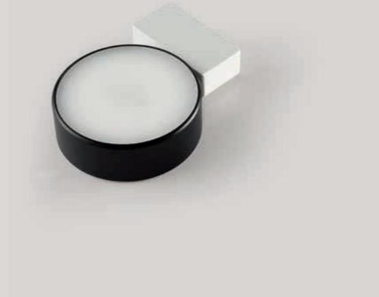
[En] → Lighting fixture in carved solid aluminium, powder-coated available in 4 colors and concrete finish. White PMMA diffuser. LED 220-240V. 359° adjustable version as wall/ceiling lamp. Frame in powder-coated aluminium, available in 4 colors. Chromed metal joint.
