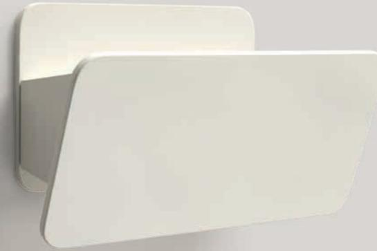
[En] → 5 mm thick powder-coated front metal reflector, available in 4 colors. RAL 9010 back reflector and side bands powder-coated white RAL 9010. The LED lighting source 220-240V is installed in the middle of the lighting fixture and generates a double light emission controlled by the tilt of the frontal reflector.
