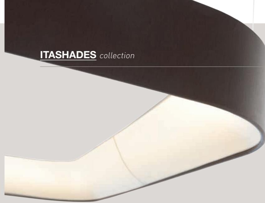
[En] → Unit composed by: outside shade in opaque PVC completed with cotton fabric available in 7 colors. Inside shade in transparent PVC completed with white cotton fabric. Prismatic PMMA cover. Strip LED 20W/m 24V.
